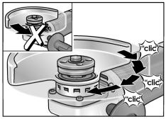
Turn guard hood opposite to the direction-of-rotation arrow on the gear head to the required position.
