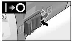
To switch off the power tool, release the switch rocker by pressing the rear end.
