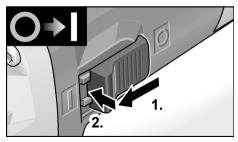
Push the switch rocker forwards (1.) and engage by pressing the front end (2.).
