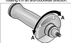
Rotate the cover on the handle by 180° until it engages. The stop key is released.
