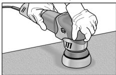
Apply light pressure to the polishing tool and make circular, overlapping movements on the surface to be polished in order to achieve good polishing results and to prolong the service life of the tool.
