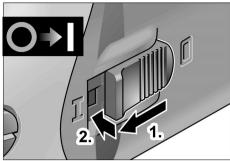
Push the switch rocker forwards and engage by pressing the front end.
