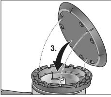
Align securing holes and fit new Velcro pad (3.).
