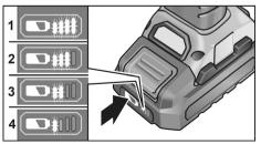
he indicator goes out after 5 seconds. If one of the LEDs flashes, the battery must be recharged. If none of the LEDs light up after the button is pressed, the battery is faulty and must be replaced.
