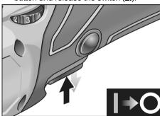
■ To switch off, briefly press and release the switch.
