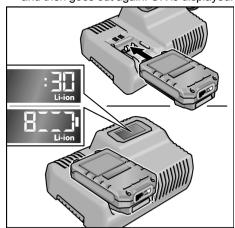
Insert the battery fully into the charger until it clicks into place.
