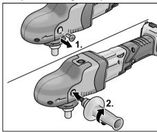
To do this, remove the handle cover fastening screw from the side on which the handle is to be attached.
